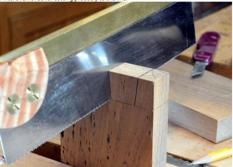
Fixture removed for cutting precisely to the line.
