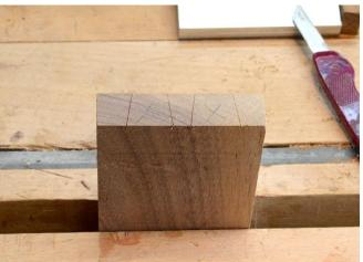
• The optimal location of the positive guide slot to the knife-mark for a tight fit is shown below. This is appropriate for pins or tails. I "split" the knife mark or move the tool slightly away from the line, towards the waste area, for a good interference fit. In case work, it may be necessary to ease up on the tightness as several dovetails (12" - 24") make fitting tight joints very difficult. Again, experiment to find the sweet spot depending on the fit you want and the wood you are using.
