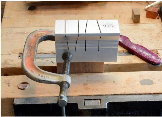
• There is no front or back side of the tool. The tail and pin slots are symmetrical from one face to face. I turn the tool or the board if necessary when I feel there is a more stable way of securely holding the fixture during cuts. I've found that it is typical to make all the cuts without having to turn either the tool or the workpiece.
